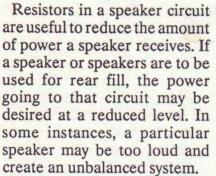
Tweeters and other small speakers may need protection and usually can afford a reduced amount of power. A single speaker used for center imaging may have both the right and left channel input to it and, in most instances, resistors are necessary to stabilize the load an amplifier sees in that section.
